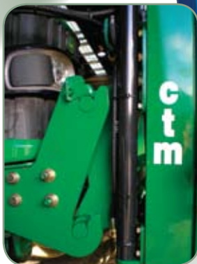
Compact Tilt Mechanism including quick detach
